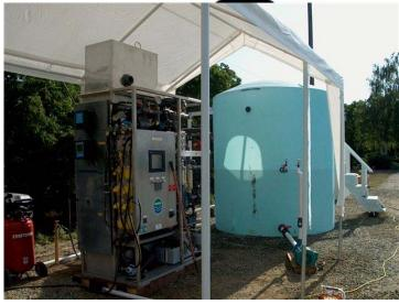
flux rates in an MBR application, and significantly reduced waste biosludge production. However we also established a clear dependent relationship between the amount of power applied per unit volume and the amount of sludge reduction. It was necessary to know this relationship at various power densities before the technology could go to the market place and designs made and performance warranties offered. *Wastewater Experts* defined a final series of tests to define that relationship.
